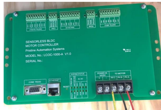
Conductor Cable Termination on Controller
