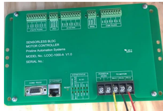
Conductor Cable Termination on Controller
