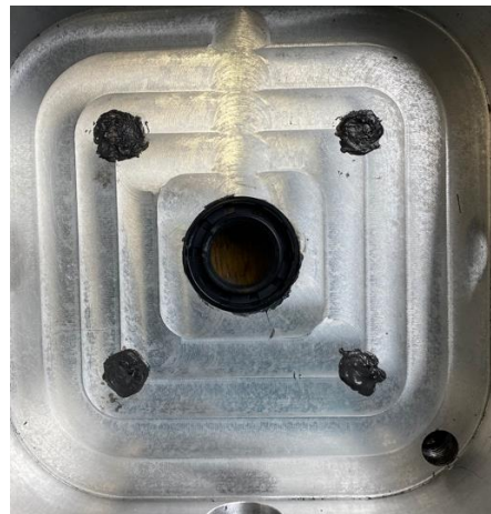
Figure 17: Shaft seal installed in topworks
