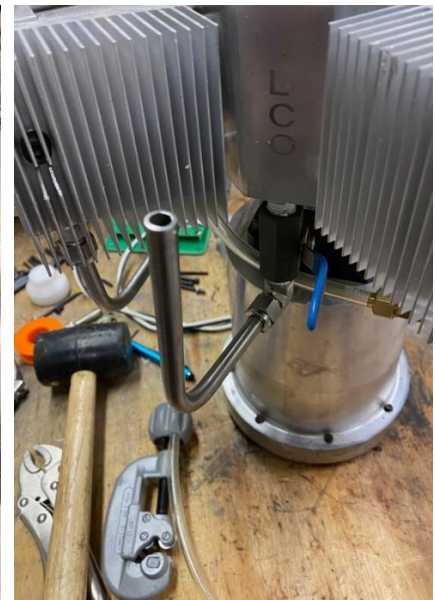
Figure 44: Elbow pointing up
