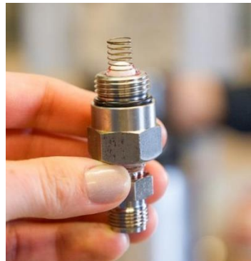
Figure 14: Bottom bushing (air inlet valve)
