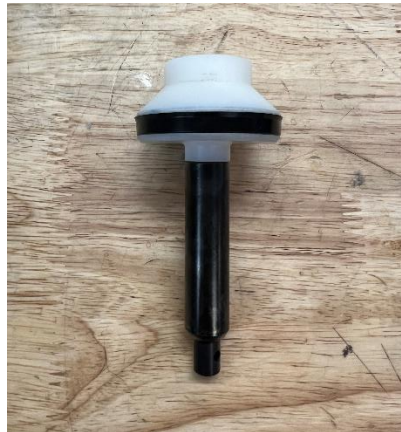
Figure 26: U-cup installed on piston
