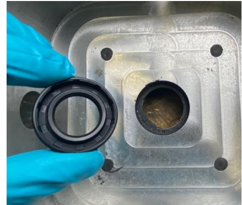
Figure 9: Remove center shaft seal
