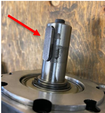
Figure 8: Remove gearbox key
