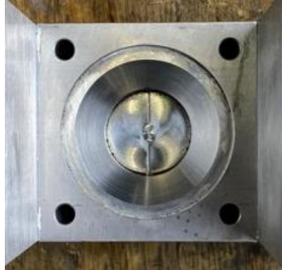
Figure 11: Clean compressor head
