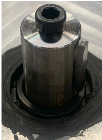
Figure 22: Insert gearbox key
