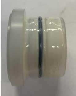
Figure 18: Sleeve with thread sealant
