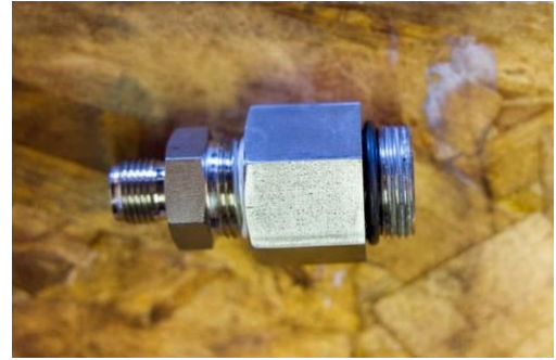
Figure 12: Remove O-ring from outlet valve (top bushing)
