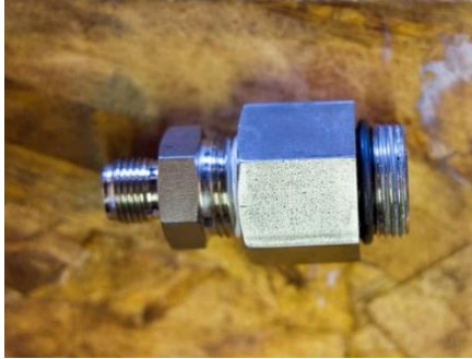
Figure 37: Installed Outlet O-ring
