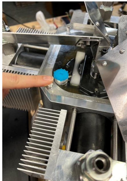
Figure 43: Replace plastic dust plug once completed
