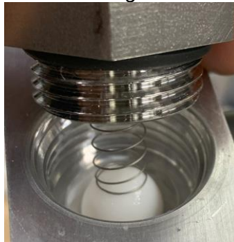
Figure 41: Installing top outlet bushing, ensuring spring is STRAIGHT
