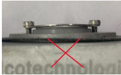
Figure 20: Incorrect – bushing plate too tight
