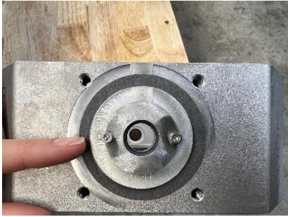
Figure 7: Remove the bushing plates & bushings
