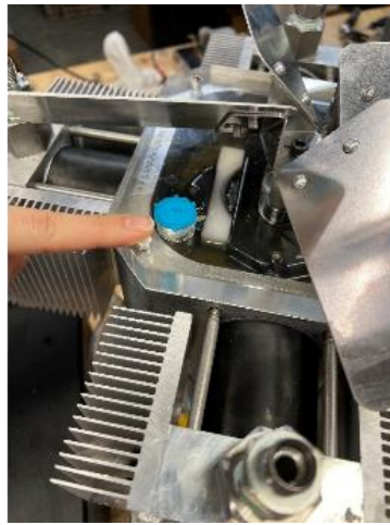
Figure 2: Replace plastic dust plug once completed
