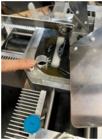
Figure 1: Hole in topworks to insert oil
