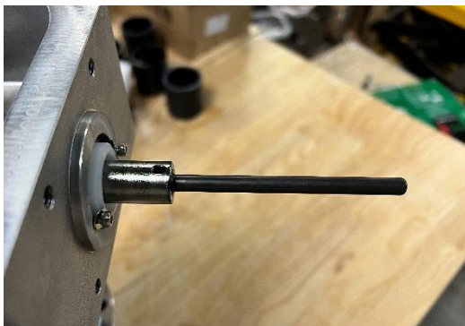
FIGURE 17: INSERT PLUNGER INTO THRUST ROD
