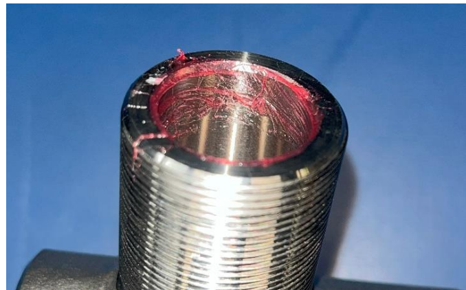
FIGURE 6: LUBE FLUID END ID
