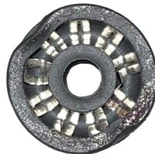
FIGURE 7: DAMAGED ONE N' DONE – DO NOT USE
