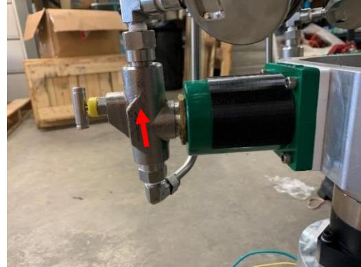
FIGURE 20: FLUID END ORIENTATION – ARROW UP
