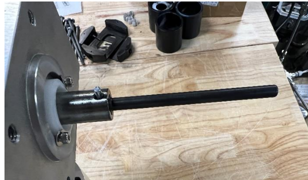
FIGURE 13: INSERT DOWEL PIN
