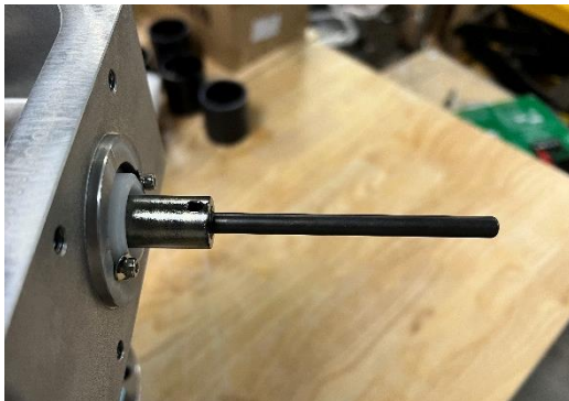
FIGURE 12: INSERT PLUNGER INTO THRUST ROD
