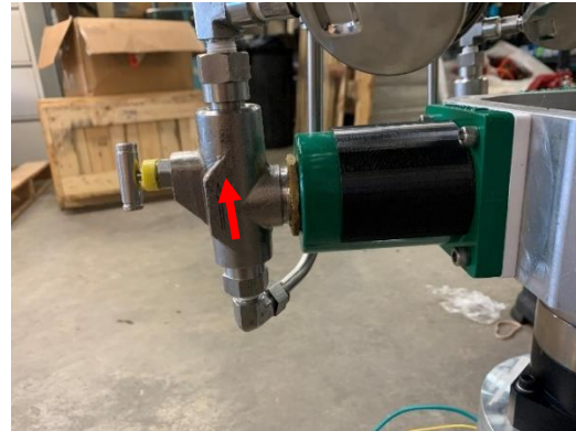
FIGURE 15: FLUID END ORIENTATION – ARROW UP
