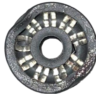
FIGURE 10: DAMAGED ONE N' DONE – DO NOT USE
