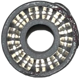
FIGURE 9: DAMAGED ONE N' DONE – DO NOT USE
