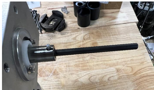
FIGURE 18: INSERT DOWEL PIN
