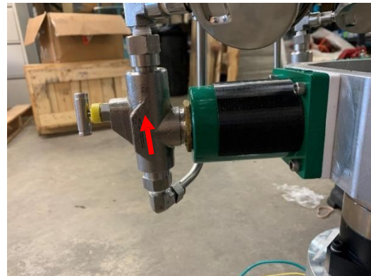
FIGURE 15: FLUID END ORIENTATION – ARROW UP
