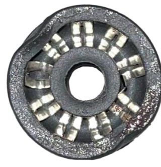
FIGURE 10: DAMAGED ONE N' DONE – DO NOT USE
