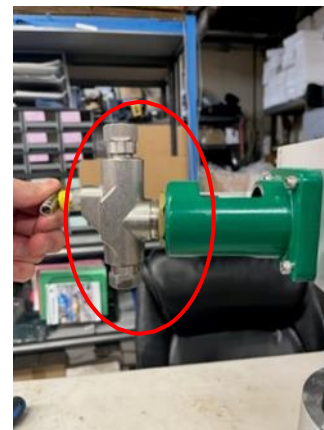
FIGURE 18: FLUID END ARROW POINTING UP
