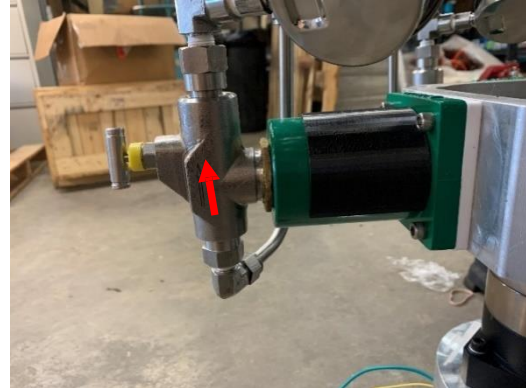
FIGURE 20: FLUID END ORIENTATION – ARROW UP
