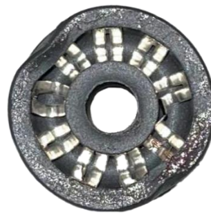
FIGURE 7: DAMAGED ONE N' DONE – DO NOT USE
