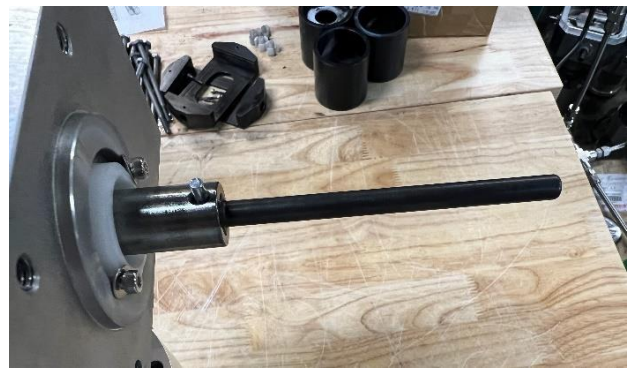
FIGURE 18: INSERT DOWEL PIN
