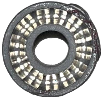
FIGURE 6: DAMAGED ONE N' DONE – DO NOT USE
