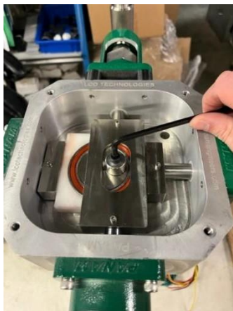
FIGURE 16: MANUALLY ROTATE 360 DEGREES WITH ALLEN KEY
