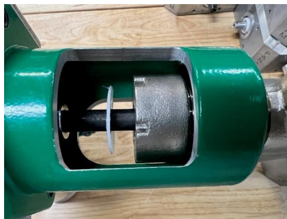
FIGURE 21: PLUNGER DISC ON PLUNGER
