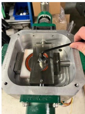
FIGURE 16: MANUALLY ROTATE 360 DEGREES WITH ALLEN KEY
