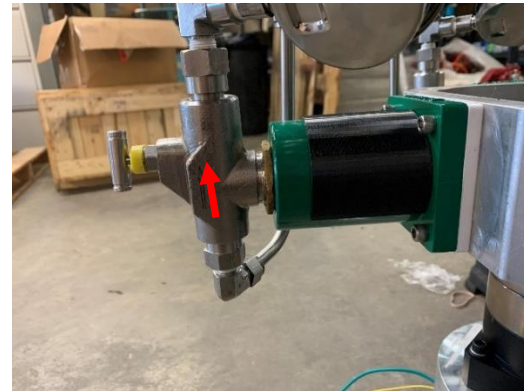
FIGURE 15: FLUID END ORIENTATION – ARROW UP
