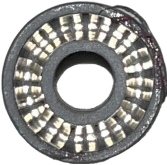
FIGURE 9: DAMAGED ONE N' DONE – DO NOT USE
