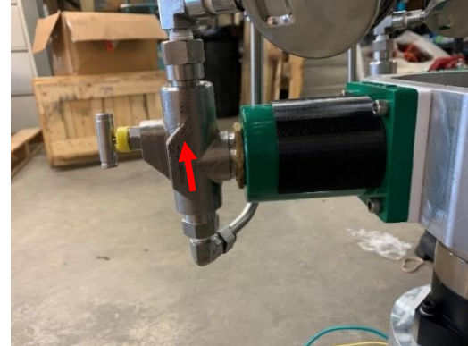
FIGURE 20: FLUID END ORIENTATION – ARROW UP
