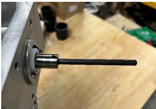
FIGURE 17: INSERT PLUNGER INTO THRUST ROD
