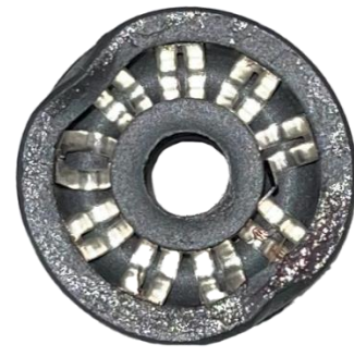
FIGURE 10: DAMAGED ONE N' DONE – DO NOT USE
