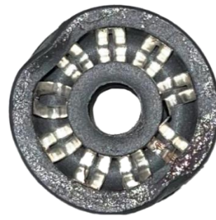
FIGURE 7: DAMAGED ONE N' DONE – Do NOT USE
