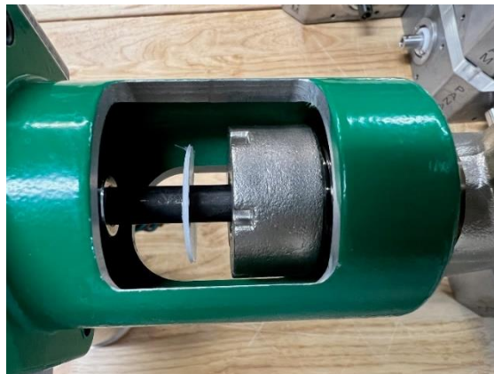
FIGURE 21: PLUNGER DISC ON PLUNGER
