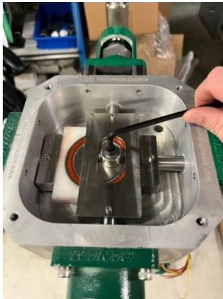
FIGURE 22: MANUALLY ROTATE 360 DEGREES WITH ALLEN KEY
