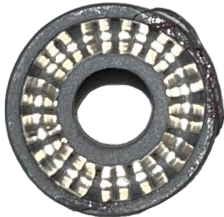
FIGURE 6: DAMAGED ONE N' DONE – Do NOT USE
