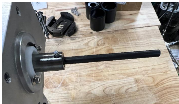
FIGURE 18: INSERT DOWEL PIN
